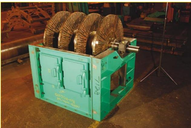
**Figure 4. L-Series feeder during assembly.**
